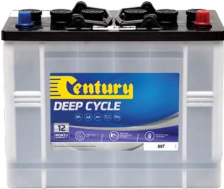
Century Deep Cycle Flooded batteries are constructed using thicker plates, specialist antimonial lead alloys and denser active material, to withstand repeated recharge and discharge cycles. The maintainable design enables easy access and topping up of electrolyte levels for maximum control over battery life. Premium grade raw materials and electrolyte ensure reliable deep cycle performance in recreational and commercial applications.
