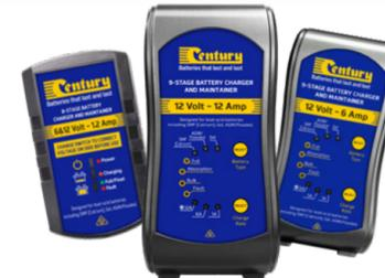
Century's range of 6 volt & 12 volt battery chargers can charge batteries rated up to 240Ah<sup>8</sup> and maintain batteries rated up to 360Ah. Incorporating patented rejuvenation technology, the chargers have the ability to recover heavily discharged batteries, and will activate from as low as 3 volts<sup>8</sup>.
